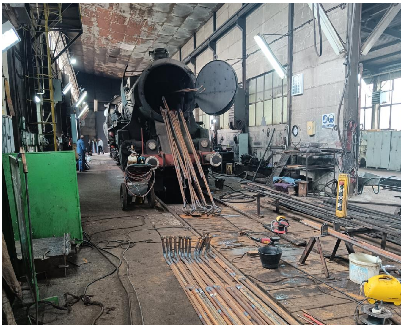
A Bosnia class 33 sits in the shed in Tuzla awaiting the refitting of its superheater elements on 24/4/24. Photo: Ian Leigh
