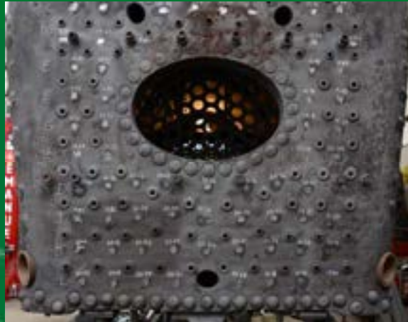
SVF- 880.001 Boiler and firebox hole after tubes removal
